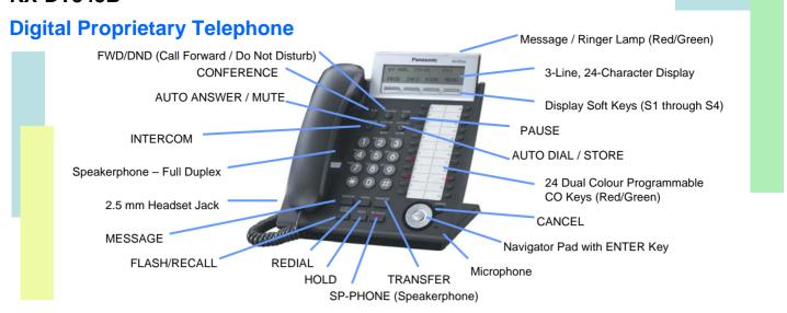
This ergonomically designed KX-DT343 Digital Proprietary Telephone offers a host of state-of-the-art functions to meet the needs of the demanding customer. A full set of control keys allow access to frequently-used functions such as transferring and conferencing calls. The Navigator Pad provides speed and efficiency when programming names and telephone numbers, searching of quick-dial numbers and use of the many other system features.
